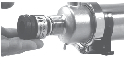
Step 4 – Remove Gland Nut From Each End
