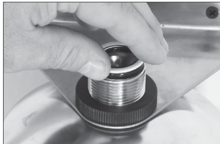
Step 5 - Place Teflon® washer over quartz sleeve until it rests on O-Ring
